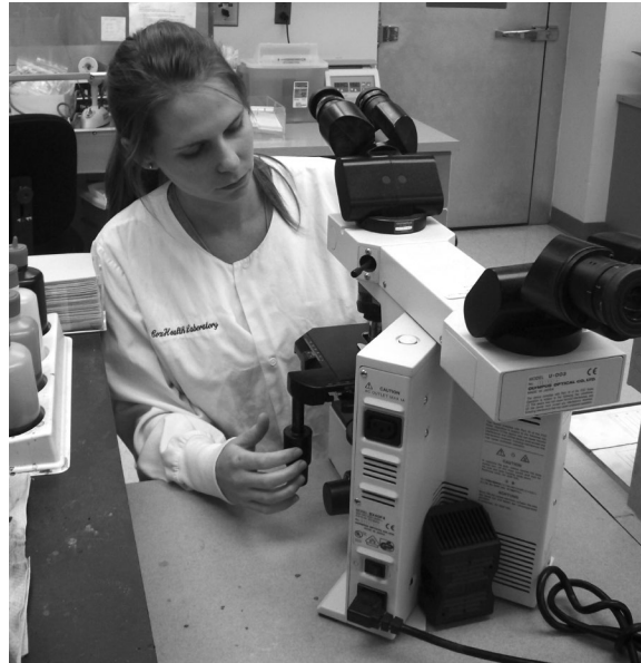
Figure 1.3 When adjusting the microscope, the technologist observes the objective carefully to prevent breaking the slide and damaging the objective lens of the microscope. This dual-view microscope has two microscope heads combined for simultaneous viewing and is extremely useful for teaching purposes. ©Verna Morton
